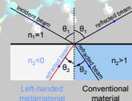
In such a material the light is refracted on the same side of the normal on entering the material (Snell's law for  $n_2 < 0$ :  $n_1 \sin \theta_1 = n_2 \sin \theta_2$ ).
