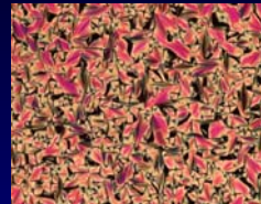
Smectic A phase displayed by compound 2 at 146°C.
