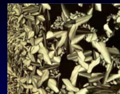
Rectangular columnar phase displayed by compound 8 at 145°C.
