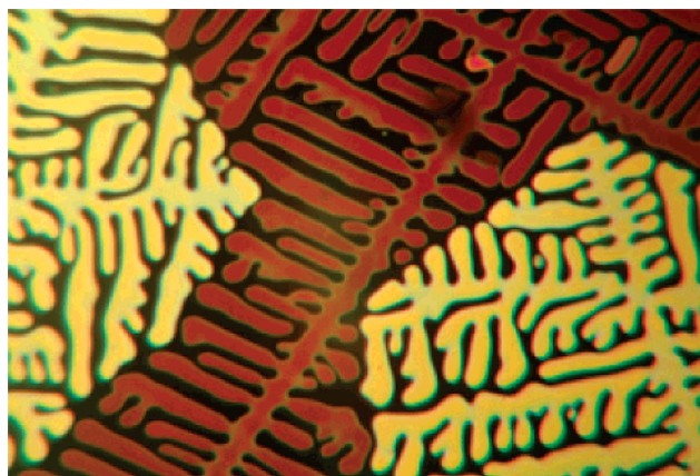
Figure 3. Representative optical textures of the three-dimensional body-centered tetragonal mesophase of 11 at 147^\circ\text{C} obtained by cooling from the \text{Col}_h mesophase.
