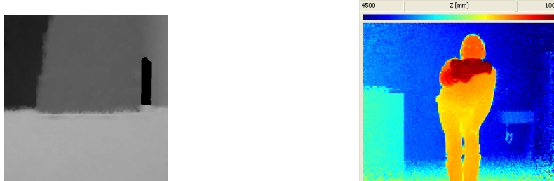
(a) 3D microscope range map - Caliper part (b) SwissRanger range map - Indoor scene
