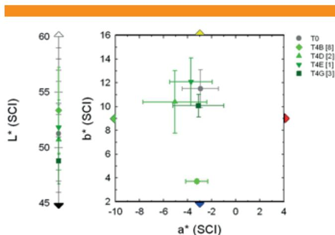
Figure 1: Colour comparison for different application methods used for the biological treatment. Values in square brackets in the legends are the  $\Delta E^*$  values respect to T0.
