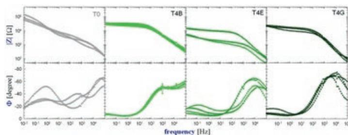
Figure 2: EIS spectra on copper urban natural coupons without treatment (T0) and with the biological treatment according to different application methods.
