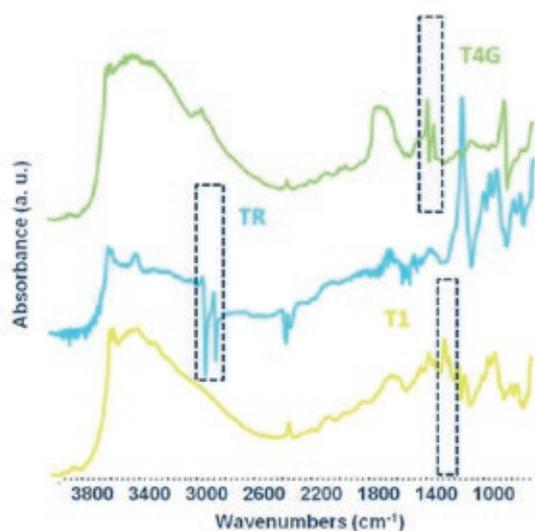
Figure 3: Reflectance FTIR spectra obtained from treated CUN coupons (urban patina) at zero months of exposure. QQ coupons (marine patina) presented the same characteristics bands for the different treatments under study (data not shown).
