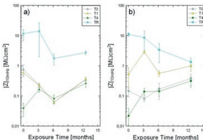
Figure 4: Average  $|Z|_{10MHz}$  values measured at zero, three, six and twelve months of exposure on QQ and CUN samples treated with none (grey), T1 (yellow), TR (blue) and T4G (green).
